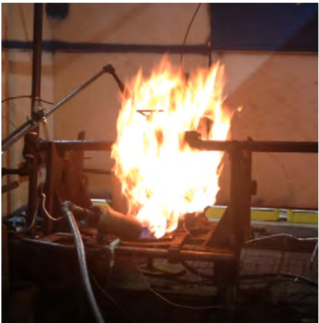
Fire test per API Spec 607 4th Edition.
